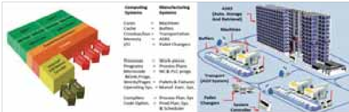
Figure 7.10 Analog of distributed manufacturing systems with PCs (courtesy of P. Ferreira, University of Illinois Urbana-Champaign).
